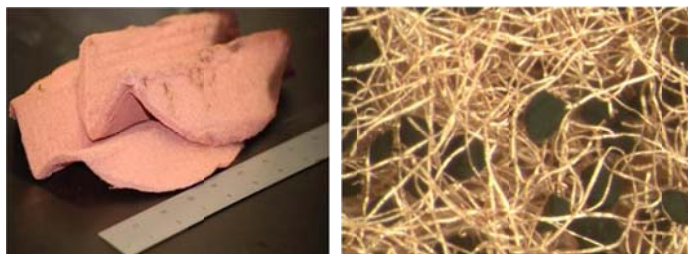
Figure 1. Left: Copper (12 \mu\text{m} ) microfibrous media (MFM). Right: 60-80 mesh particles entrapped in Cu MFM.
