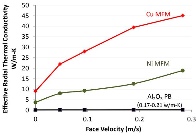
Figure 2. Effective radial thermal conductivity of Cu MFM, Ni MFM, and Al<sub>2</sub>O<sub>3</sub> Packed Bed (PB) as a function of face velocity.
